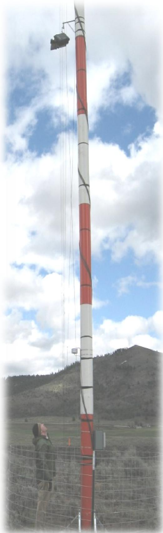
Solar-powered Anabat acoustic monitor enclosed in a weather resistant pelican case and mounted on a meteorological tower.
